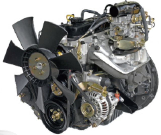
WANFENG 491GP Displacement 2237 cc Rated output: 41 kW/2800rpm Rated torque: 161 N-m/2000rpm
